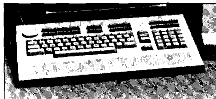
The 98203C Nimitz keyboard with the rotary knob (on HP 9000 Series 200 Model 216)
